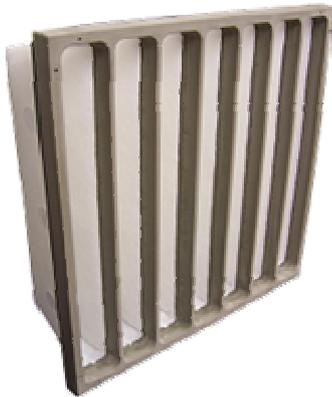
The **G-4 Pocket Filter** comes in standard 24" x 24" x 7" size (8 pockets) or sized to fit the EMW VK-KW System (7 pockets). It has a high dust holding capacity and low pressure drop. It has no metal parts and comes standard with an all plastic frame that is fully incinerable. The **G-4 Pocket Filter** uses
